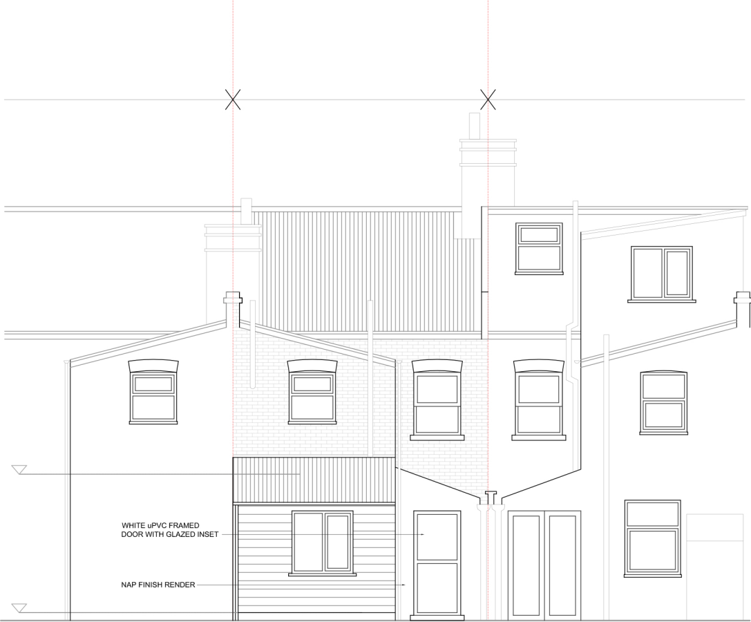
PROPOSED REAR ELEVATION SCALE 1:100
